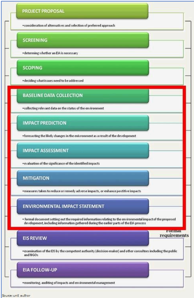
Figure 6: EIA Process stages in UK, and the stages in red square indicating some of the EIA topics use as Good Practices categorization.
